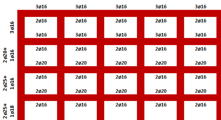
Fig. 5.2. Reinforcement of the beams and columns (side reinf.), existing 4 storied structure
