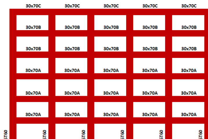
Fig. 4.3. Dimensions of the frame elements, 6 storied structure
